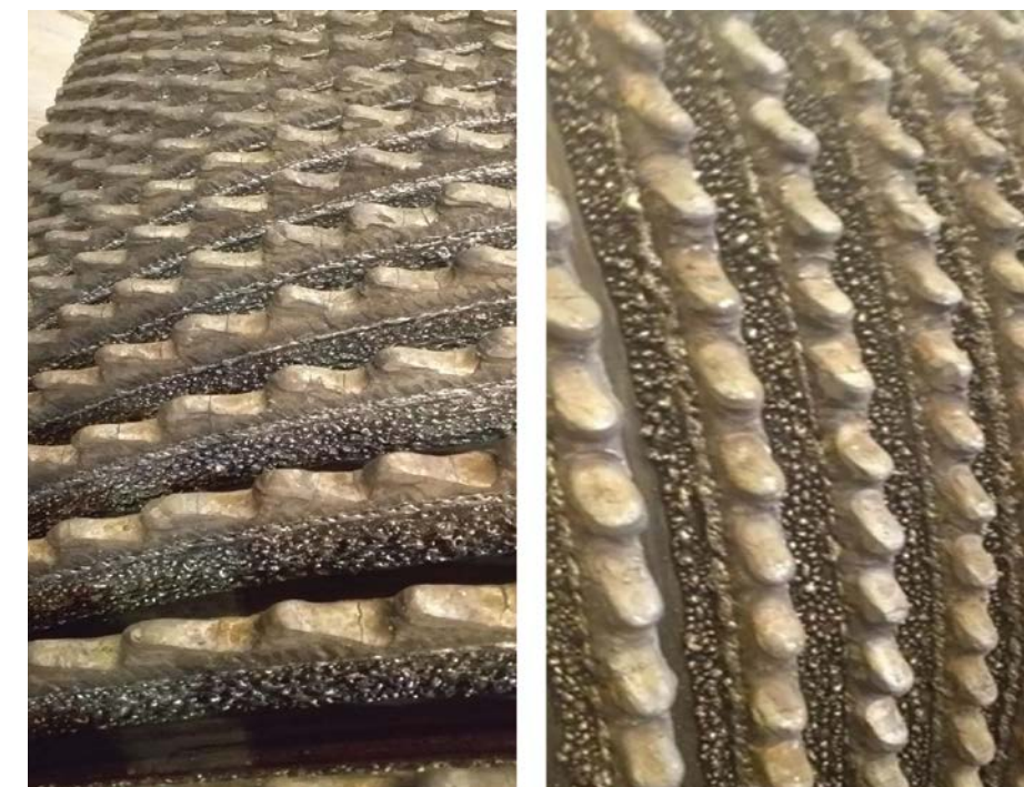
On the left, the new UTP Vanadium SG consumable for roller arcing produces a sharper grip with more arcing material than the original UTP Vanadium 500 consumable on the right. This not only enhances the wear resistance of the crusher rollers but also improves the sharp grip, which leads to increased production efficiency.
