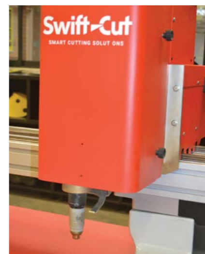
The Swift-Cut system features Intelligent Torch Height Control. The torch height is set automatically through voltage sensing, so the plasma arc is always at the optimum height for the cut.
