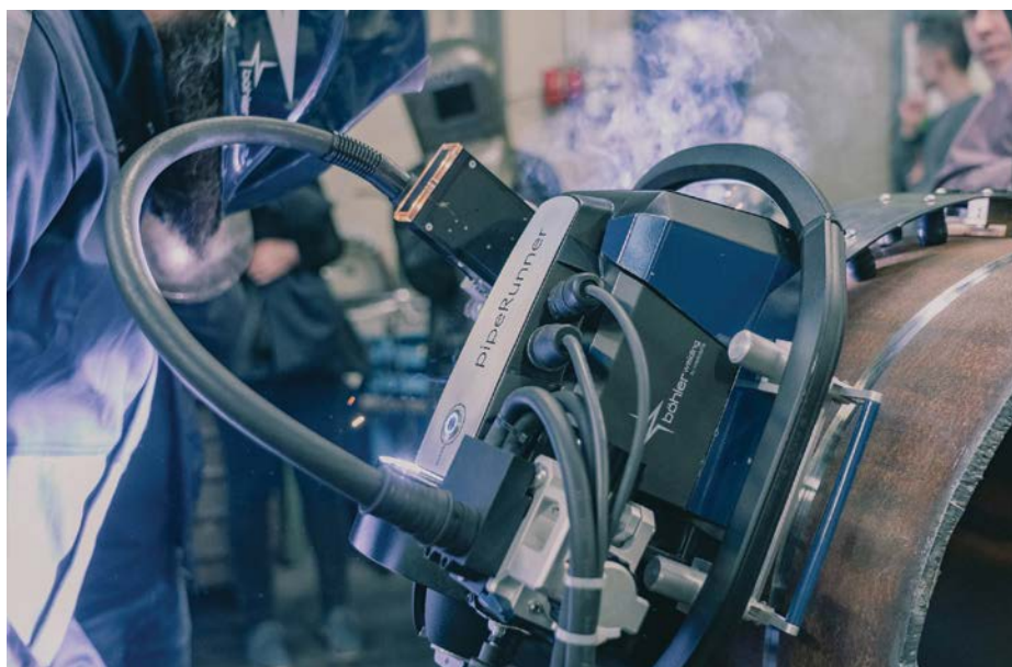
pipeRunner® is designed for pipeline and process piping girth welds for carbon steel to corrosion resistant alloy (CRA) materials.
