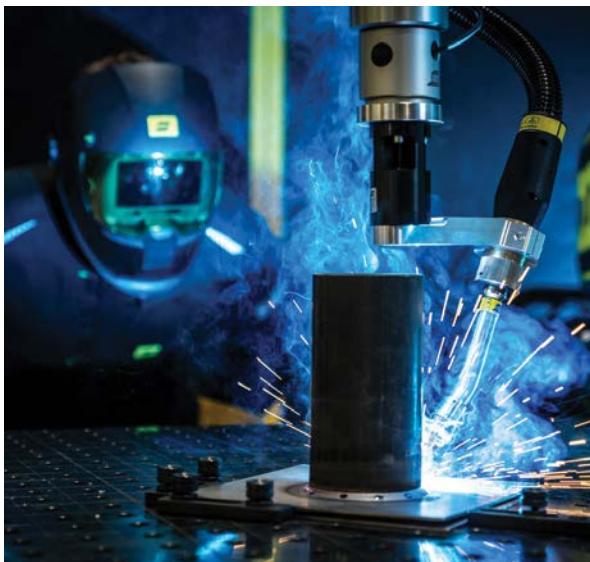
Collaborative robots (cobots) are easy to program and ideal for high-mix, low-volume work in small- to medium-sized fabrication shops.
