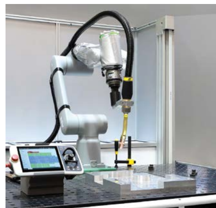
ESAB UR10e COBOT is a fully self-contained, small-footprint and mobile robotic MIG/MAG welding system.
