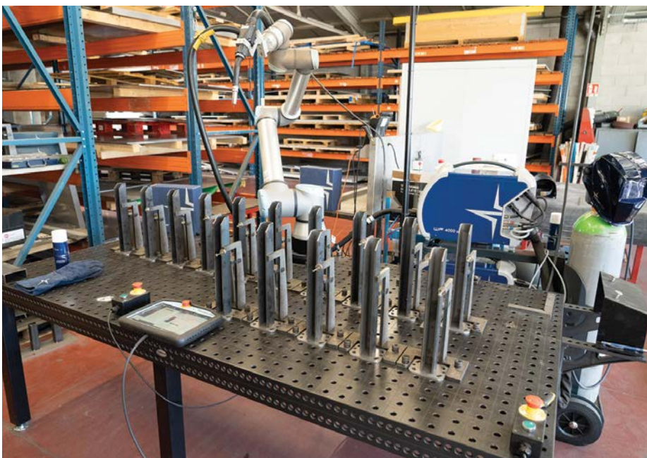
Böhler Welding's CO-BRO® collaborative robotic solution, using the Uranos NX 3200 GSM welding power source, is in use, welding 250 to 400 brackets per day.
