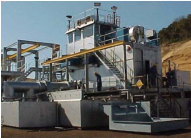
A dredger manufactured and supplied for suctioning material from rivers or sea beds and sending heavy mineral concentrate directly to processing or separating plants.
