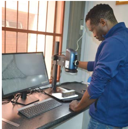
Walter Mahlangu sets up SAIW's high-definition digital microscope and measurement system to analyse weld test samples.
