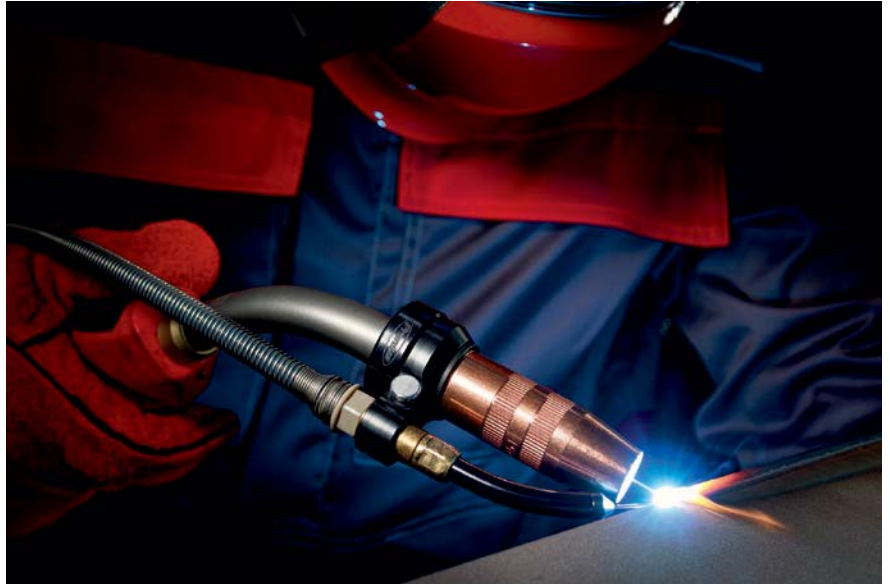
The Velo wire 'pushes' the torch along the weld to maintain a constant welding speed and a constant contact-tip-to-workpiece distance.
