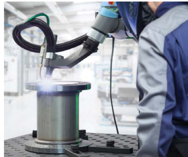
CO-BRO® FLEX from voestalpine Böhler Welding is a high-tech workstation for robotic collaborative MIG-MAG welding.
