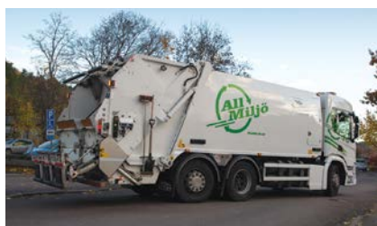
For Scania recycling and waste-disposal trucks in Sweden, Hardox® HiAce steel is now being used to extend the life of truck bodies.
