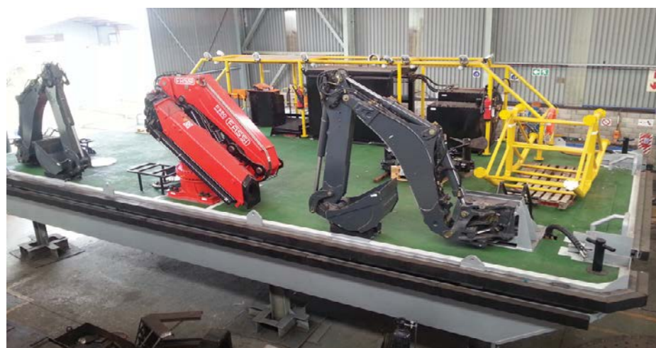
A GENMAC-manufactured and supplied barge equipped with two back actors, a crane for loading and offloading plant equipment, a full hydraulic system and a Z-Drive for propulsion.
