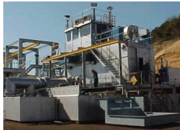
A dredger manufactured and supplied for suctioning material from rivers or sea beds and sending heavy mineral concentrate directly to processing or separating plants.
