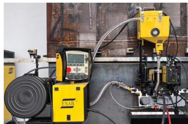
ESAB AGW1 series of tank welders is the best yet for 2G welding construction in jack-up fuel tank construction.
