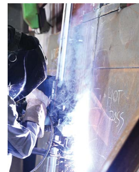
When using the railRunner mechanised solutions with a flux-cored wire, the time to completion is only 49 min, compared to 468 min with SMAW, which is nearly 10 times faster.
