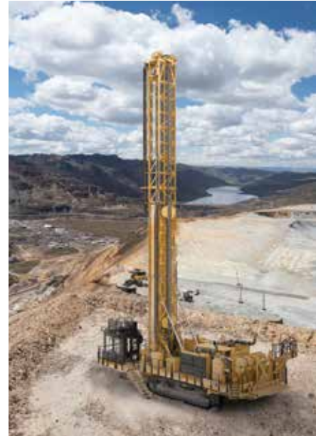
The MD6380 is capable of pull-down force of 49 895 kg and rotation torque of as much as 20 880 Nm.
