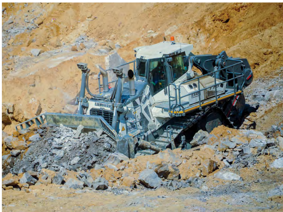
The principal benefit of a hydrostatic transmission on a dozer is the absence of gears, resulting in seamless operation, uninterrupted power flow and infinitely variable speed control.
