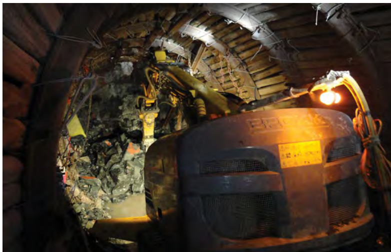
For one operation, using demolition robots to open up older shafts allowed them double monthly linear output while reducing labour requirements by 44%.
