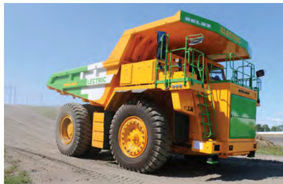
The electric mining dump truck is based on the BELAZ-7558 family, with a payload capacity of 90 t and a net weight of 76 t.
