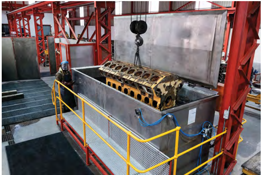
An engine block being lowered into the tank at Metric Automotive Engineering.
