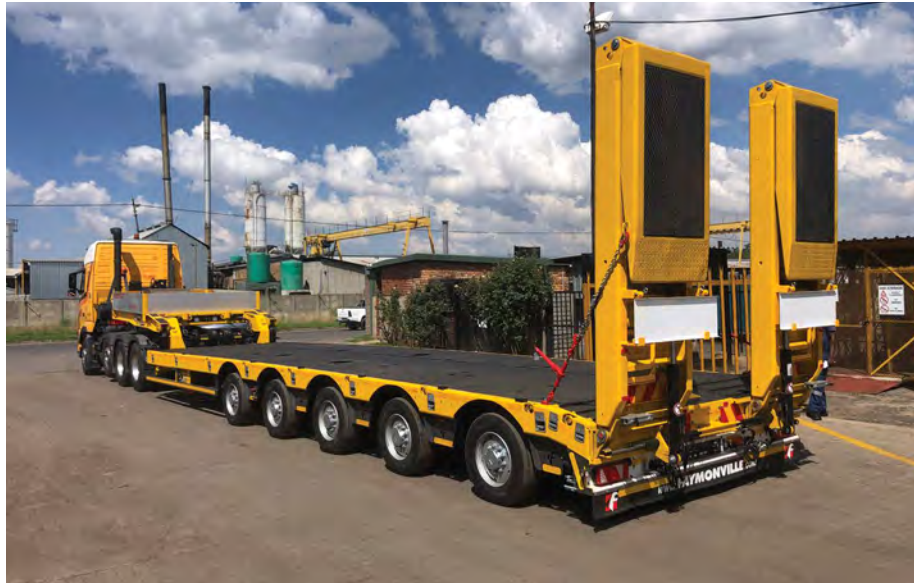
The yellow low loader with a basic width of 3 000 mm has an hydraulic gooseneck.
