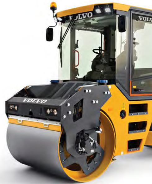
To account for the increased wear on the drum surface, the Volvo DD105 OSC roller has a hardened, abrasion-resistant alloy steel drum shell, which increases longevity.
