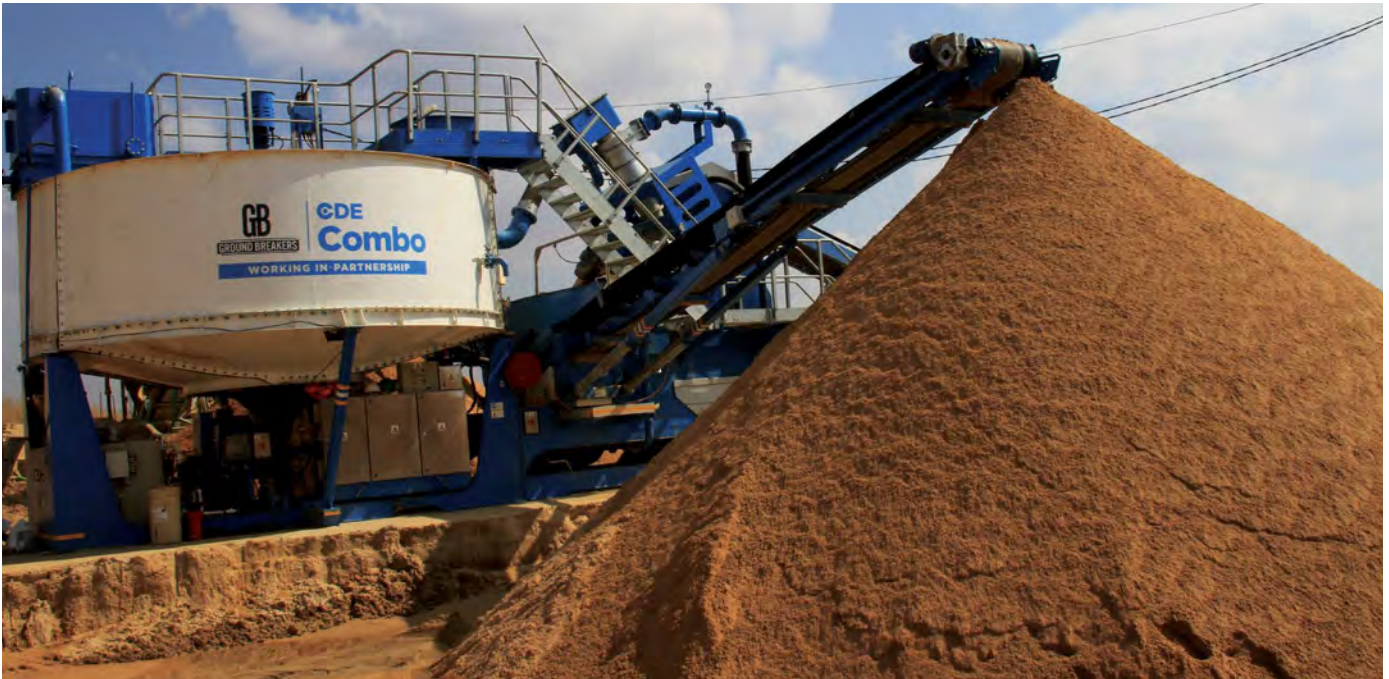
CDE developed and built a Combo modular plant to transform 60 tph of raw feed into washed 0 – 6 mm river sand and 0 – 1,5 mm plaster sand.
