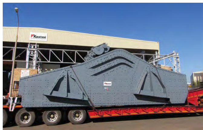
Large scalper screen leaving Kwatani for the end user in an iron ore mining application.
