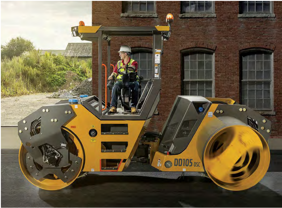
Fitted with the flexibility of the Volvo oscillation technology – which eliminates vertical vibrations – the DD105 OSC offers high compaction performance while producing a non-damaging oscillation movement.
