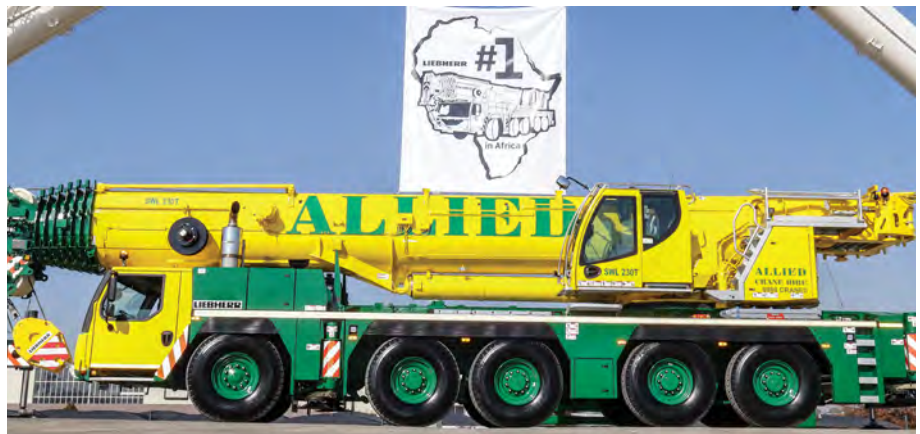
The LTM 1230-5.1 sets a new benchmark in the 230 t class with its 75 m telescopic boom.
