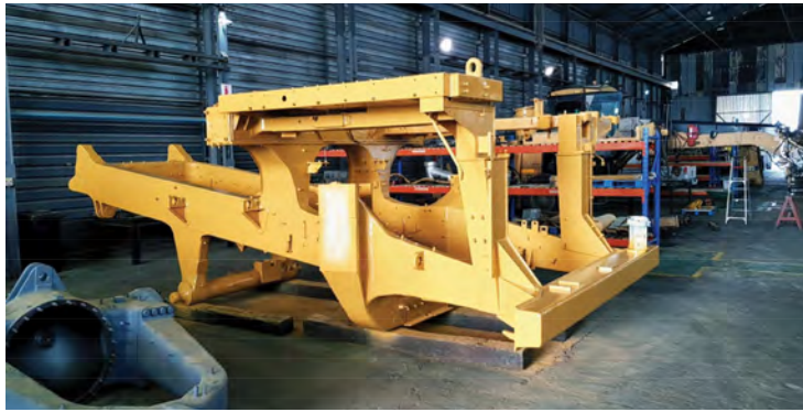
A Cat D9 dozer stripped down to its frame at the Catkom refurbishment centre.
