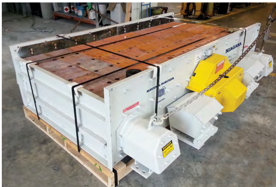
A vibrating screen after refurbishment by Haver & Boecker Niagara.
