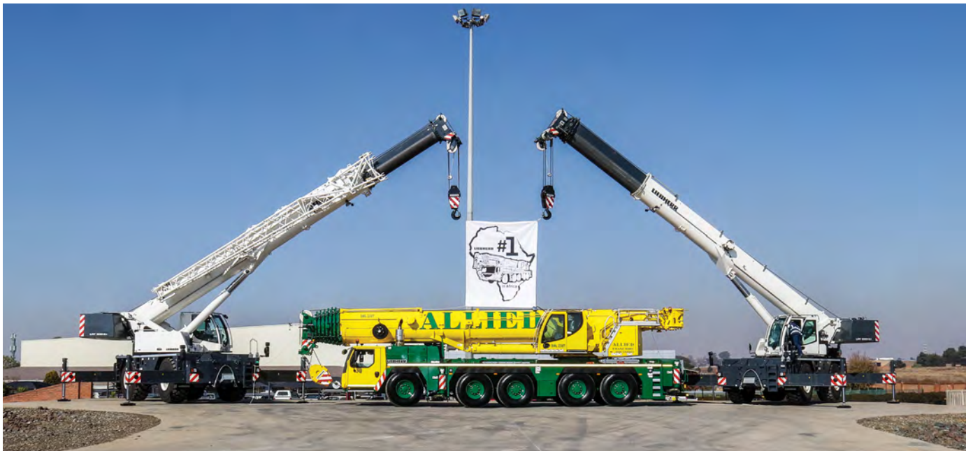
The new LTM crane is the first to have an asymmetrical support base – with the width being 7,4 m at the front and 8,1 m at the rear.
