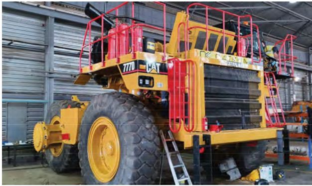
A Cat 777D off-highway truck under refurbishment by Catkom.
