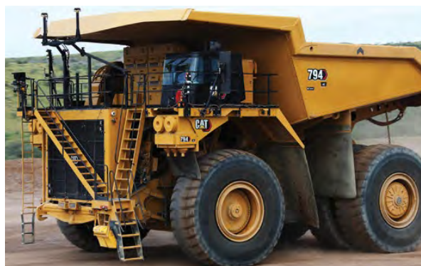
The 794 AC, equipped with Command for hauling, enables total autonomous operating of the mining trucks.
