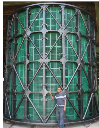
Multotec offers SAG mill trommel screens able to screen in excess of 5 000 tph on copper processing plants.
