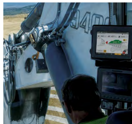
The Truck Loading Assistant helps the operator to achieve optimal truck payloads and avoid truck under- and overloading.
