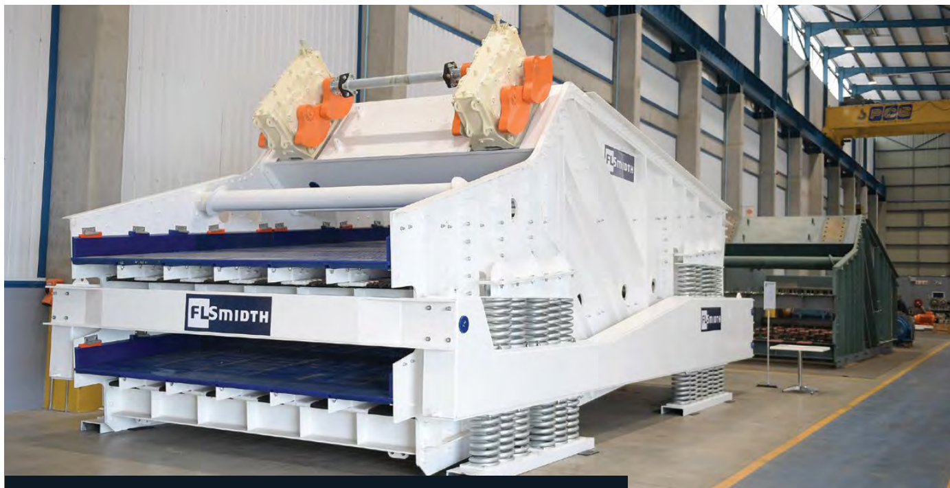
FLSmidth's double deck vibrating screen with modular panels at the company's Delmas Supercenter.
