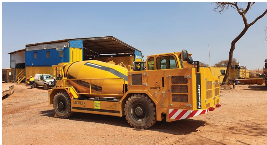
The Putzmeister MIXKRET 5 low-profile concrete transporter and mixer features an air conditioned cabin and an automatic speed regulation system.
