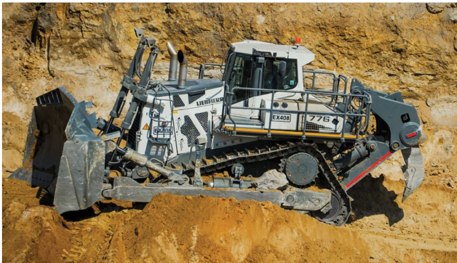
The best on offer in Liebherr's dozer range is the PR 776 – the first dozer in the 70-t class to be hydrostatically driven.
