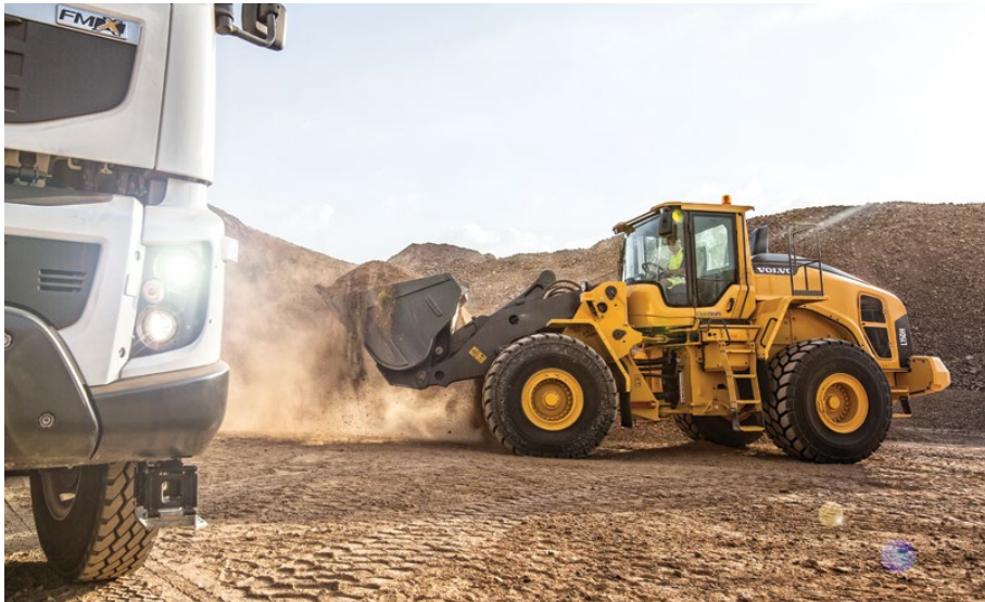
Onboard Weighing on Volvo's H-Series loaders provides real-time insight into bucket load.
