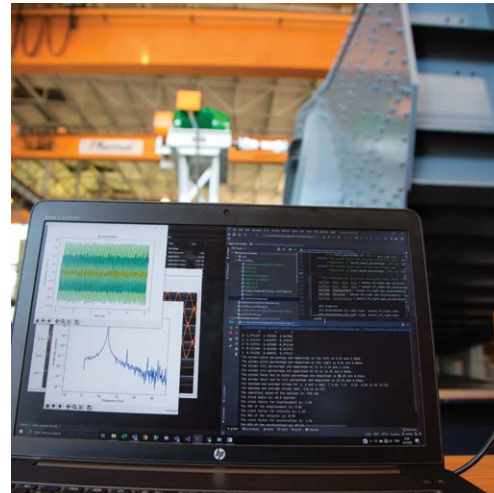
Condition monitoring on a scalper screen being tested at Kwatani.
