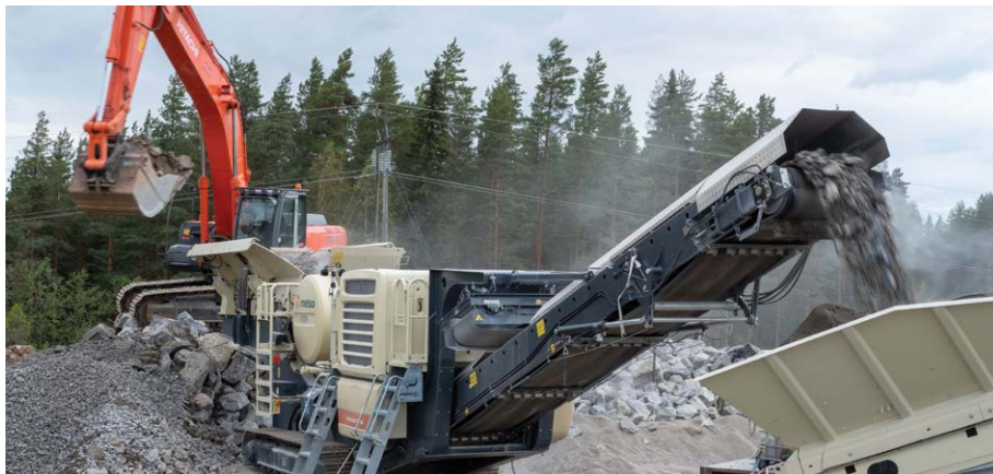
The Lokotrack® LT106™ mobile jaw crusher is often used as a primary crusher in a multistage crushing process or as a stand-alone unit and is ideal for medium-sized aggregates production, as well as recycling demolition waste such as crushing concrete.
