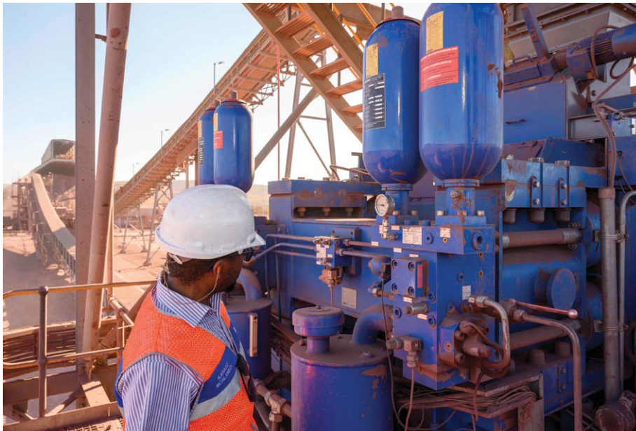
Enduron® high pressure grinding rolls can decrease energy consumption and significantly reduce water consumption.
