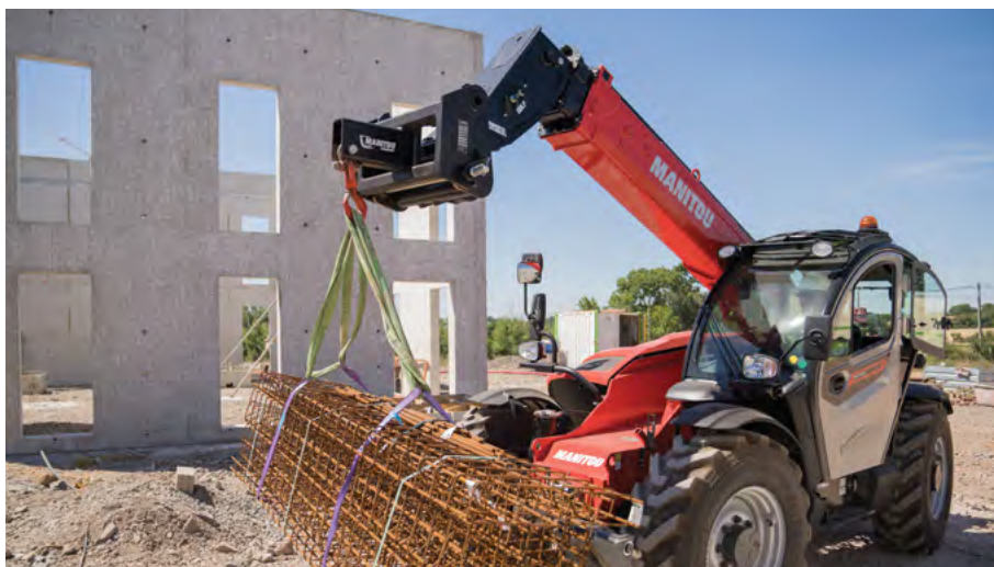
Fitted with a more spacious cab, the MT 1135 remains relatively compact with an overall width of 2,28 m, including the front stabilisers, making it ideal for use in tight spaces.
