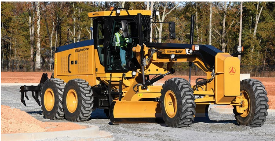
The SANY SMG200 is equipped with adjustable suspension seat, air-conditioning with heater, LED work lights and a rear camera
