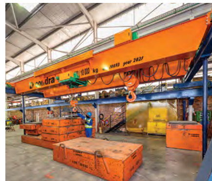
The double-girder electric overhead travelling crane is for dragline house maintenance.
