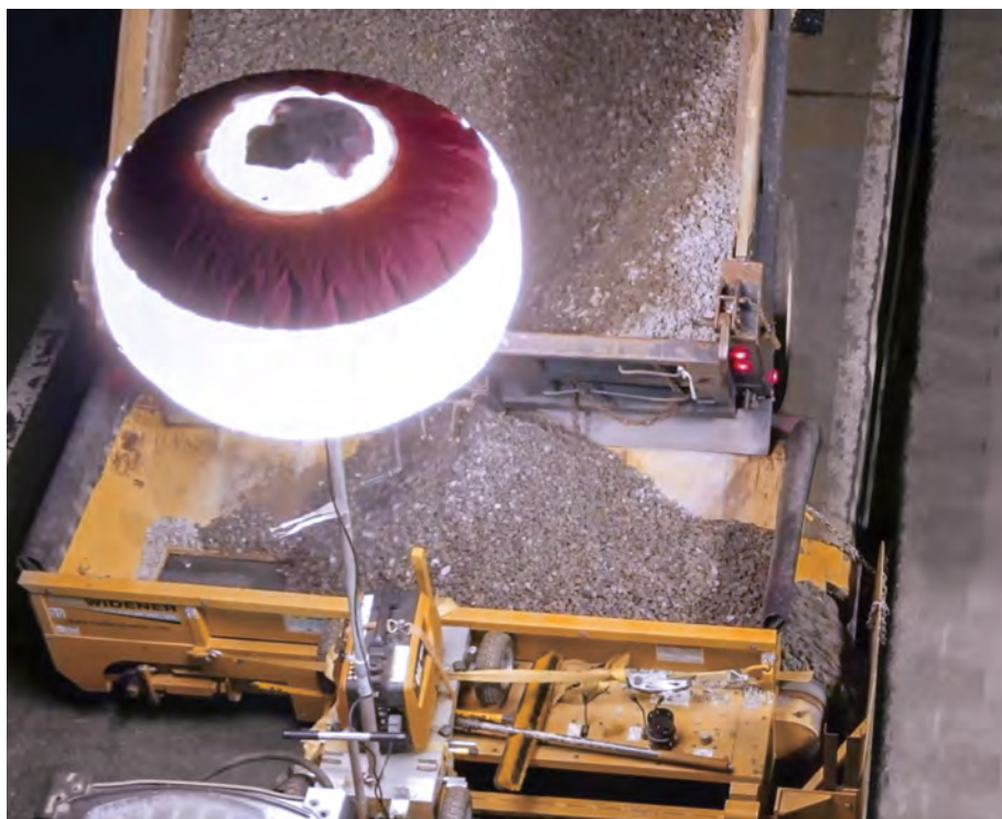
Some attachments can even dispense up to 20 t of aggregate in under 10 minutes.
