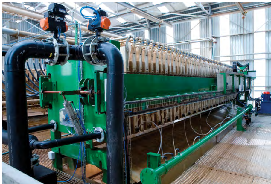
Multotec filter press recovers maximum water and produce dewatered product suitable for economical conveying to the next step or discard the waste economically.
