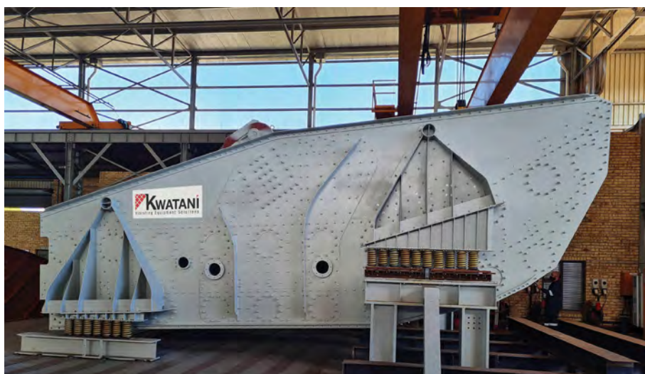
Kwatani applied its new innovative approach to the banana screen designs for a diamond mine in South Africa.
