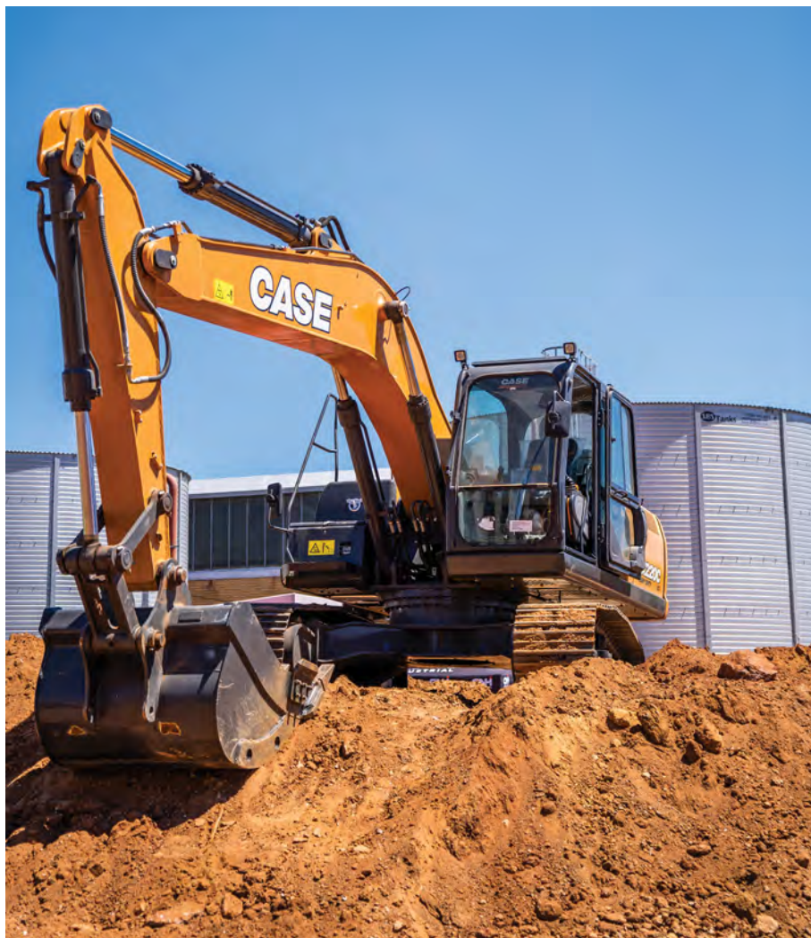
The CX 220C LC, which replaces the company's previous offering, the CX 210, is suited for a range of applications, including quarrying, forestry, roadworks, earthworks and general construction.
