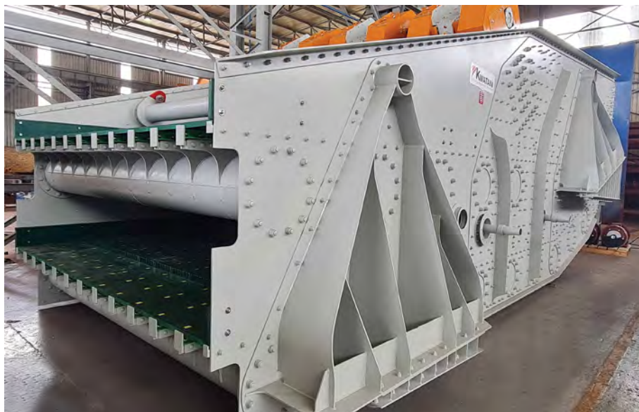
A large Kwatani double deck banana screen used in the diamond mining industry.
