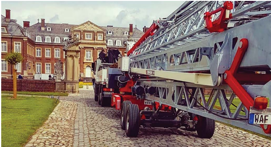
The cost of establishment and de-establishment of self-erecting cranes is very low as a mobile crane is generally not required.
