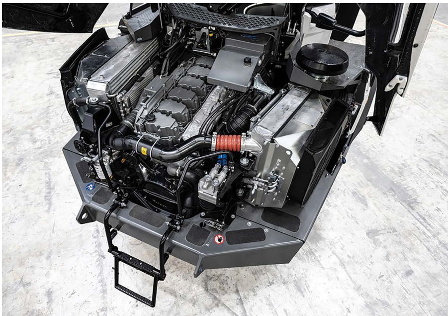
The TA 230 is powered by a 6-cylinder engine with a 12 ℓ displacement, delivering 265 kW of power
