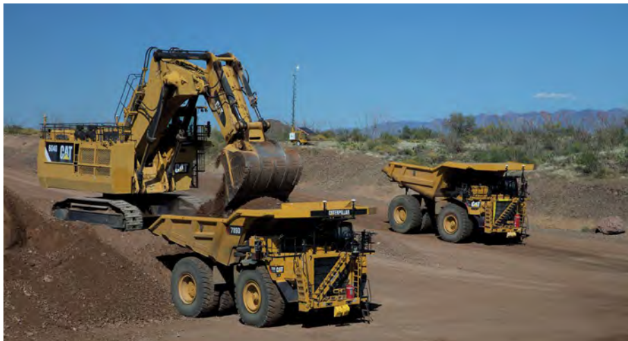
Command for hauling trucks now span class sizes from 190 to 360 tonnes.
