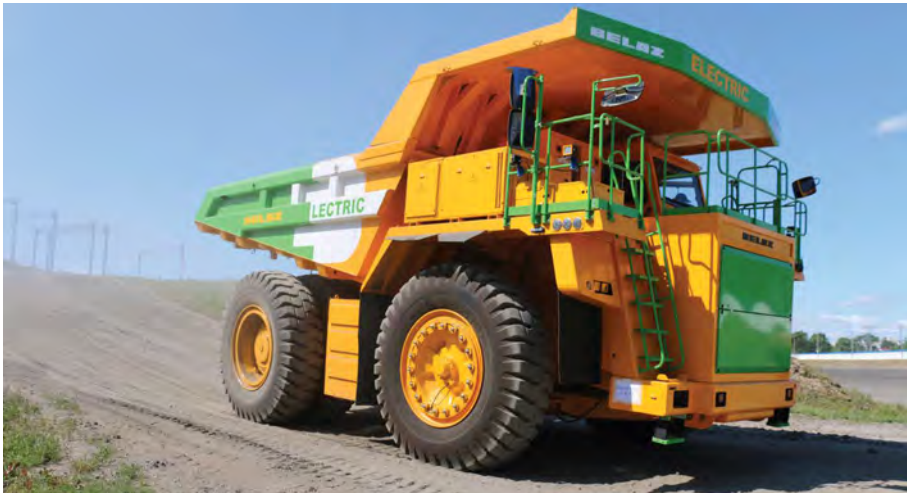
The BELAZ electric mining dump truck is based on the BELAZ-7558 family, with a payload capacity of 90 t and a net weight of 76 t.
