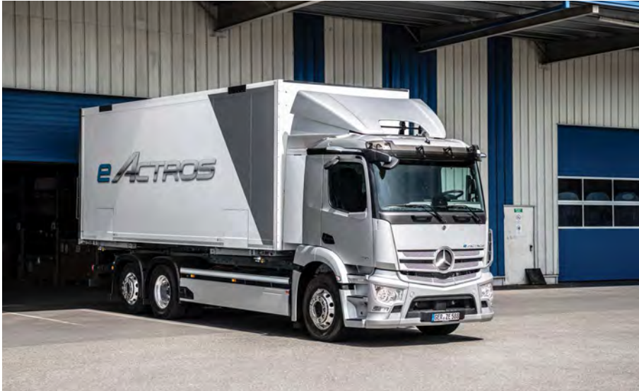
The eActros is available as a two or three-axle truck with 19 or 27 tonnes permissible gross weight.
