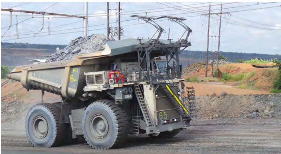
The Liebherr trolley assist system is an effective first step on the company's road to zero emission mine sites of the future.
