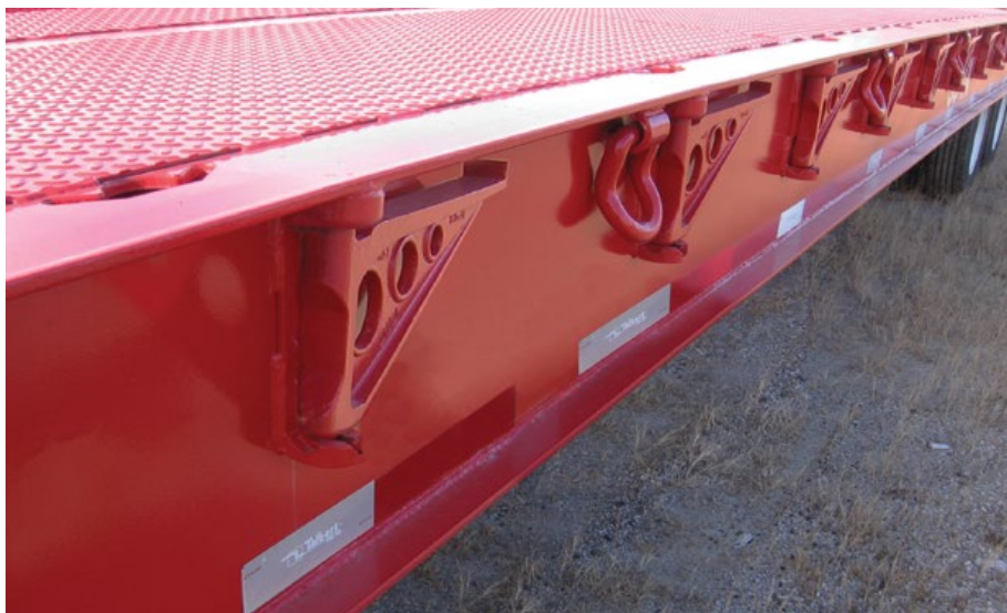
Select heavy-haul trailers made from high-strength steel, such as 12-inch deep I-beams with a minimum yield strength of 100 000 psi, for long-term durability.
