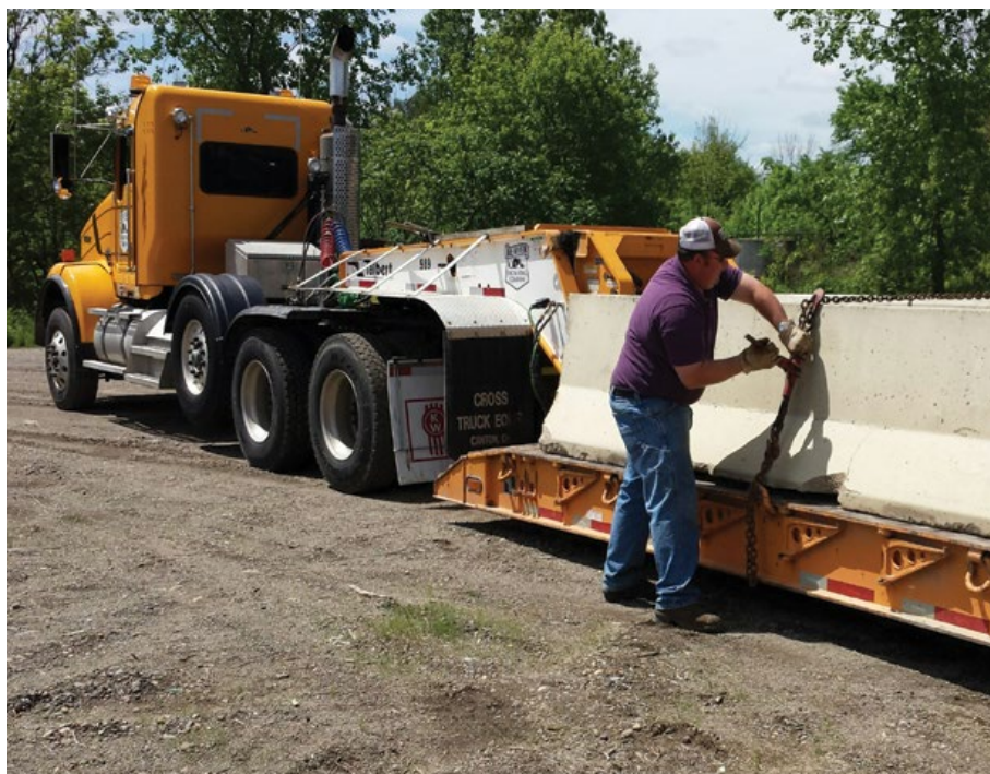
In addition to inspecting the trailer body and systems for damage, operators should double check load securements.
