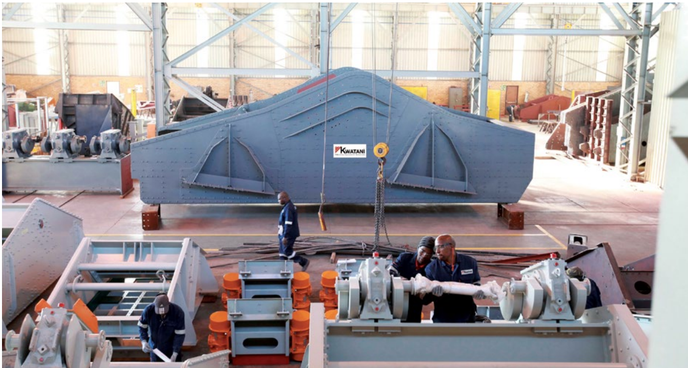
Kwatani screens, gearboxes and motors on the assembly shop floor.
