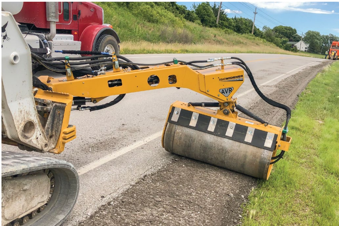
Road Widener now offers a spray bar system on its patented offset vibratory roller, thus increasing the versatility of the attachment.
