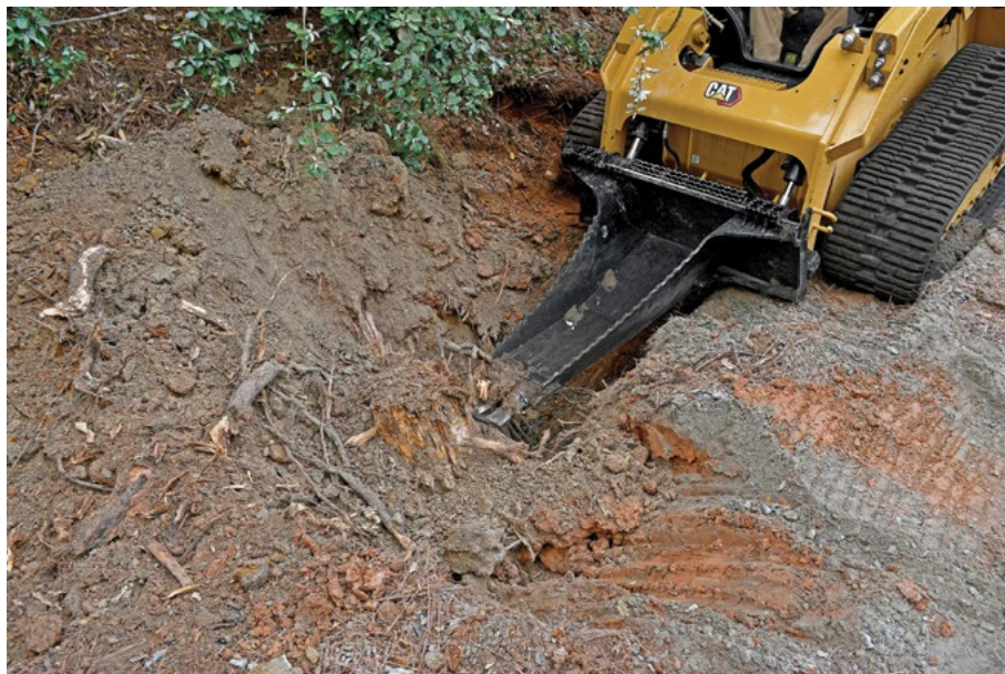
Designed for land clearing and the removal of invasive trees, stumps and large shrubs, the stump bucket is purpose designed for removing and carrying tree stumps.
