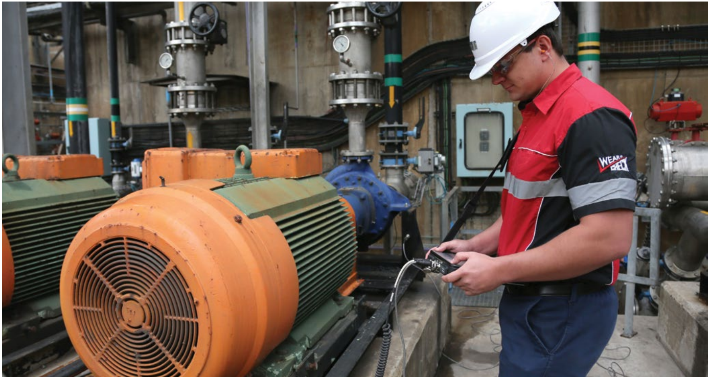
WearCheck ARC technician Peet Peacock performs vibration analysis testing.
