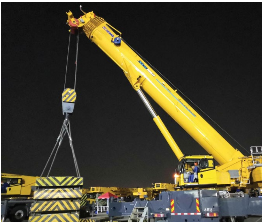
The XCA200 is noted for its 72 tonne counterweight where auxiliary winch, hook, outriggers, outrigger floats, spare tire, and the like, can be carried on board.
