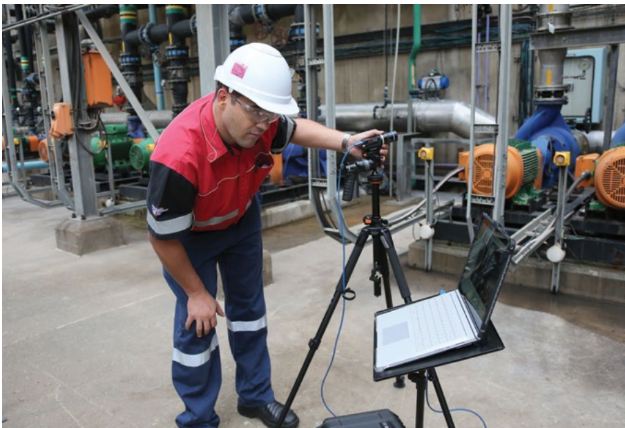
Louis Peacock, senior ARC technician at WearCheck, conducts motion video amplification testing on machinery at a water reticulation plant.
