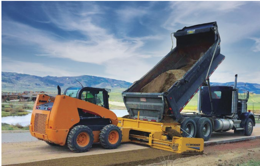
The FH-R is a versatile solution for material placement, precisely dispensing topsoil, gravel, asphalt, limestone and more – all with an attachment compatible with common machines already on the jobsite.
