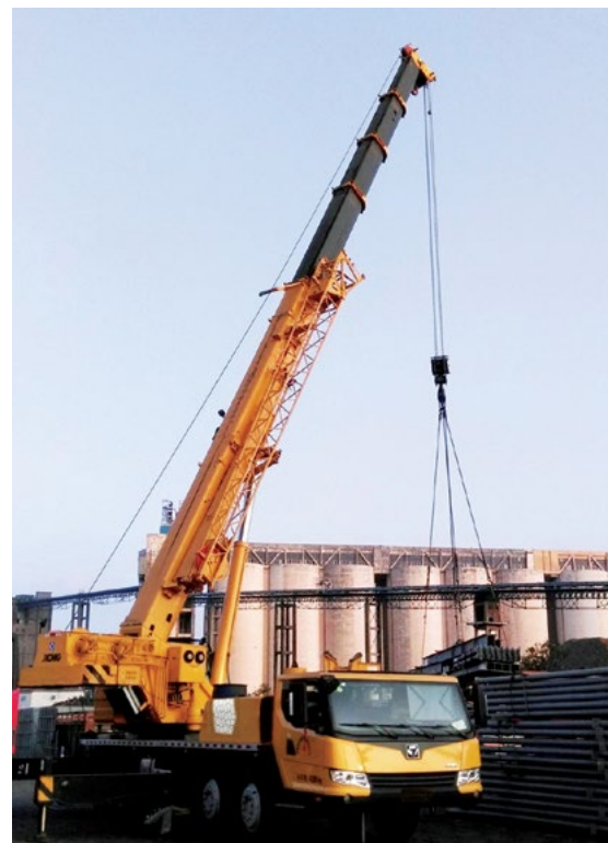
The XCT60_Y offers a maximum lifting load of 60 tonnes with the maximum lifting height at 59.8 m.
