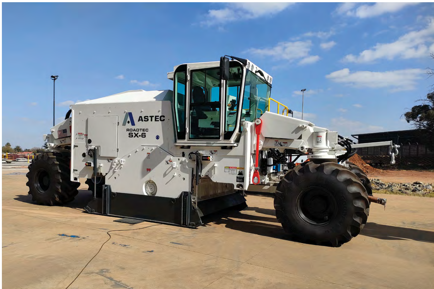
The SX-6EX's durable frame is built from strong A656 grade 80 steel, which has twice the yield strength of the mild steel in other competitor machines on the market.
