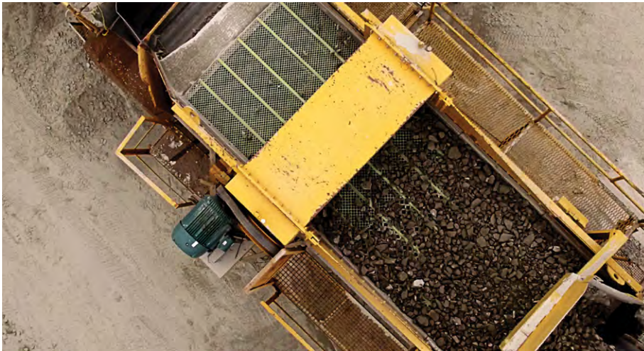
The increased screening action from high vibration screen media spreads material over the entire screen's surface area on all decks.
