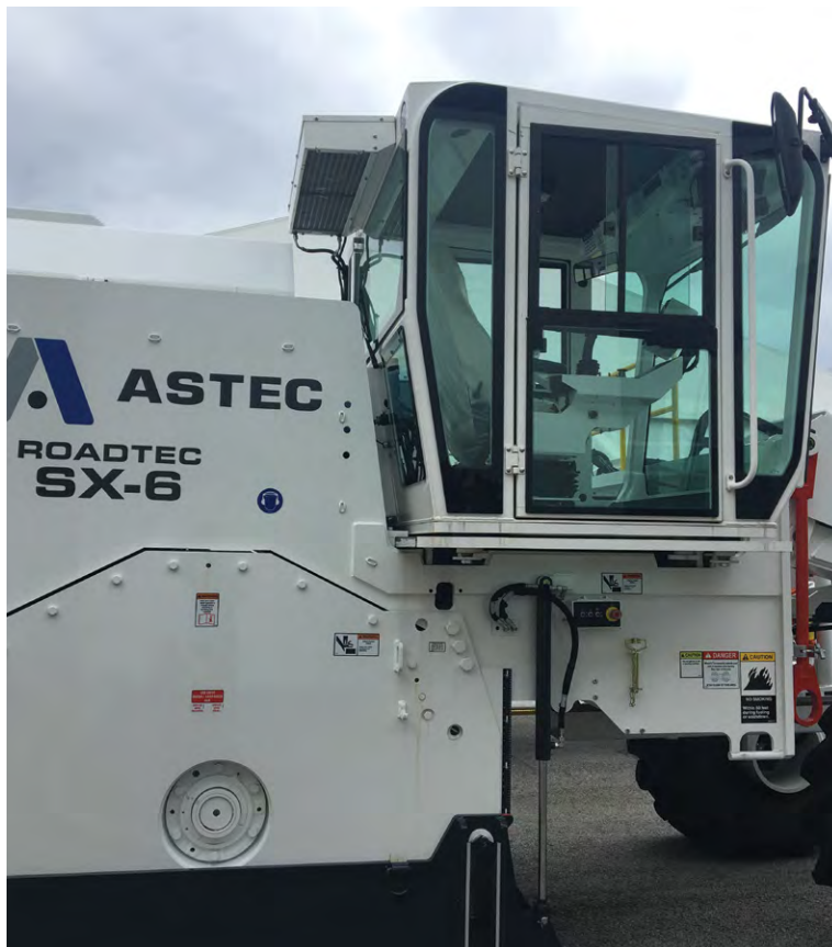
A full-view cab gives the operator an excellent view of the cutting edge and any obstacles that may be in the way.
