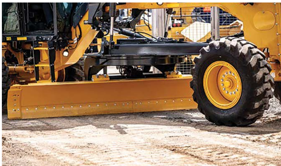
The function of graders is to prepare the road, angling it to allow for water run-off.
