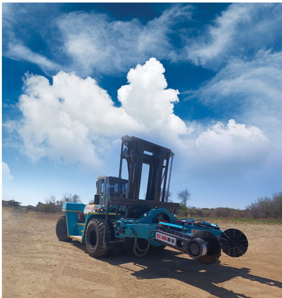
Konecranes developed a custom-built tyre handler for use in the mining industry in Chile, Australia, and South Africa.
