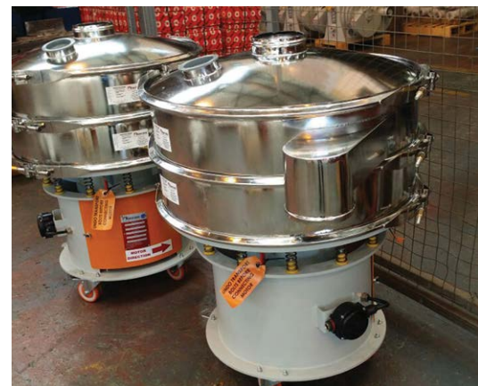
Kwatani round separators are typically used for low-volume screening.
