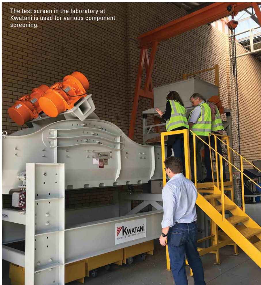
A Kwatani rectangular separator is typically used for high-volume screening.
