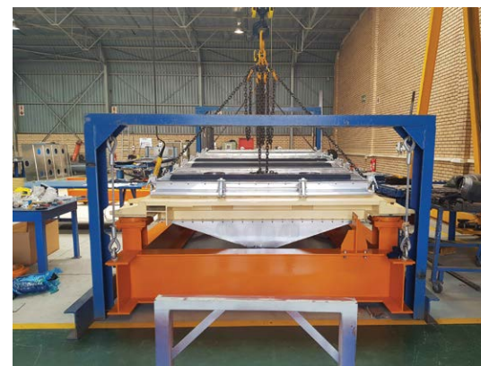
A Kwatani rectangular separator is typically used for high-volume screening.
