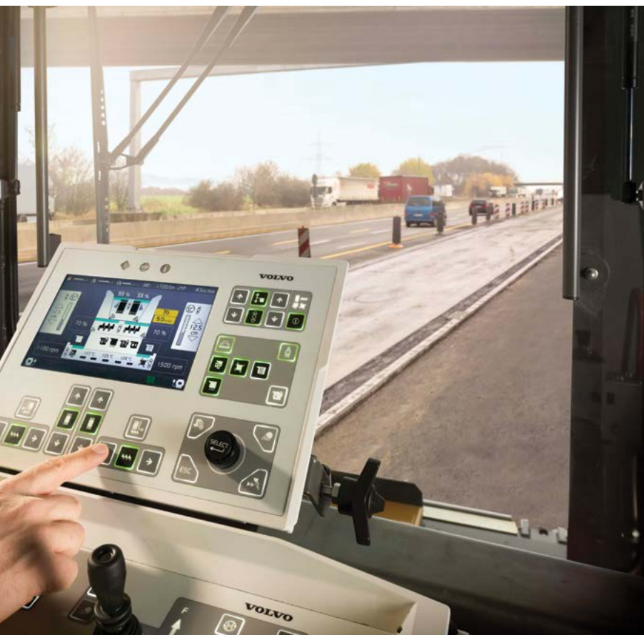
Screed status and behaviour can also be monitored by the paver operator from the Electronic Paver Management (EPM3) control panel.
