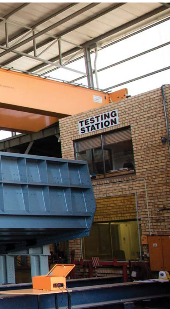
A motor driven single deck Kwatani screen for the zinc mining industry.
