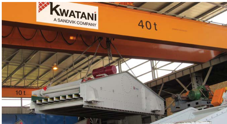
A motor driven single deck Kwatani screen for the zinc mining industry.
