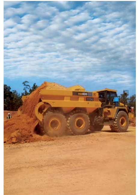
A rear-eject body offers a consistent clearance, allowing operators to safely access limited-clearance areas and maneuver around the mine. This boosts productivity for applications like reclamation, where large amounts of material need to be moved, saving valuable time and can increasing efficiency for these support tasks by up to 25%.
