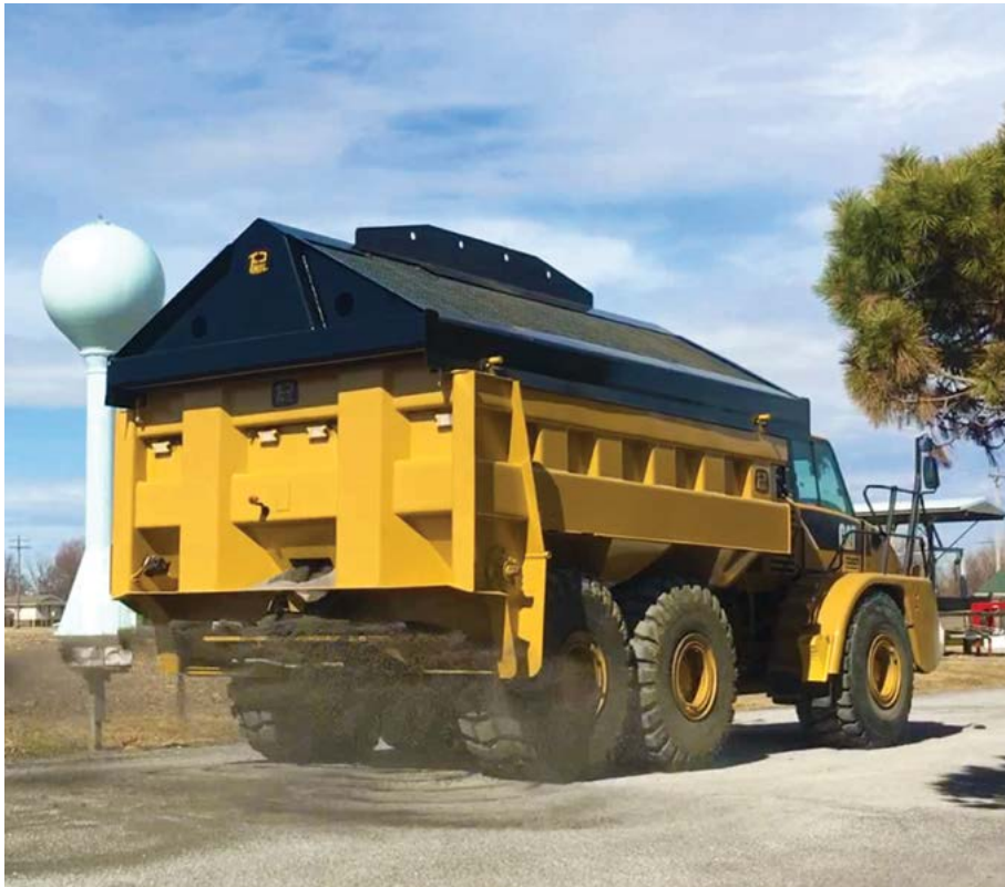
Adding a material spreading attachment to a rear-eject body provides maximum equipment versatility in every season. These attachments are available from industry-leading equipment manufacturers and are designed to integrate seamlessly.
