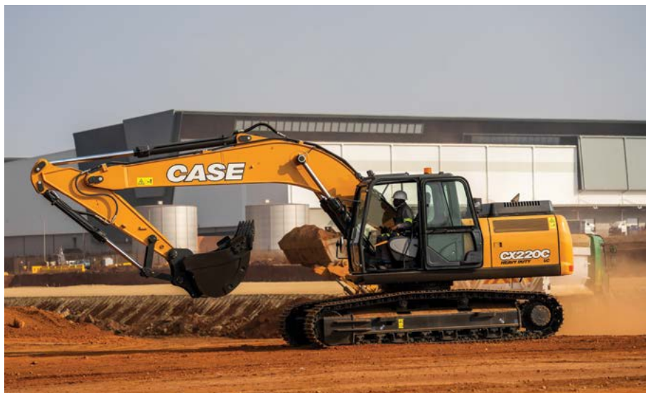
The CX 220C LC Heavy Duty excavator offers a robust design with increased plate thickness on HD structures to improve durability.
