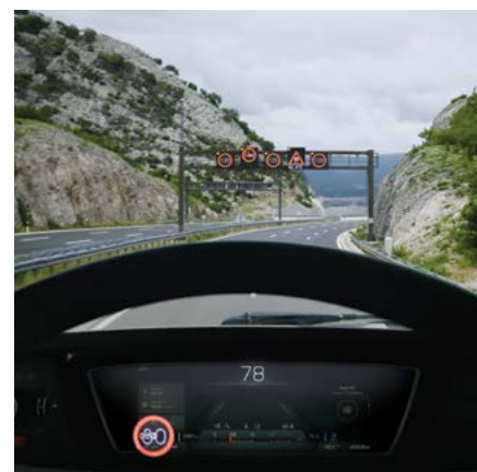
Intelligent Speed Assist (included in the GSR) keeps the driver informed about speed limits by detecting road speed signs and displaying the limit on the instrument panel.
