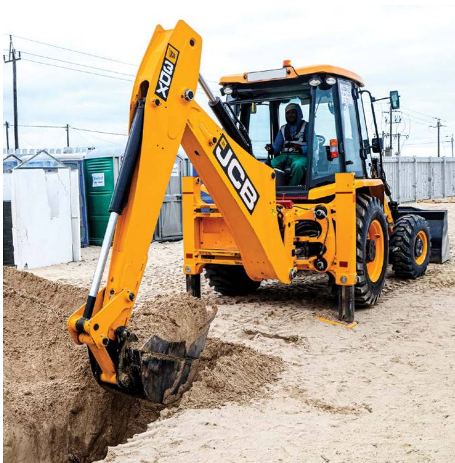
The JCB 3DX Eco's naturally aspirated 4-cylinder, 4,4 litre JCB Dieselmix 444 engine purrs along while working at the coast, which is where the bulk of Amanzi Plant Hire equipment is hired.
