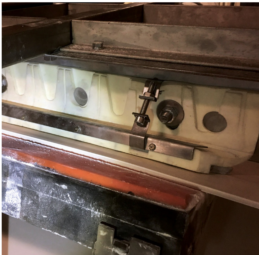
BLT World's DustScape dust filter system, which is used in conjunction with the contact-free AirScape conveyor belt skirting system, has been specially developed for the control of dust formation and material spill at critical sections along the conveyor route and transfer points.
