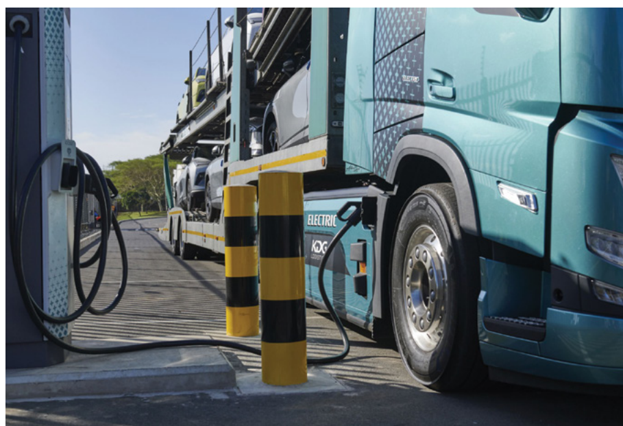
Volvo's electric trucks can be charged with an AC charger (for example a charging box) at up to 43 kW and with a DC system (stationary charging station) with a capacity of up to 250 kW.
