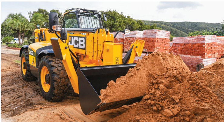
The JCB 540-170 Telehandler's stability is brought about by its mass of 12 tons and all-wheel drivetrain.
