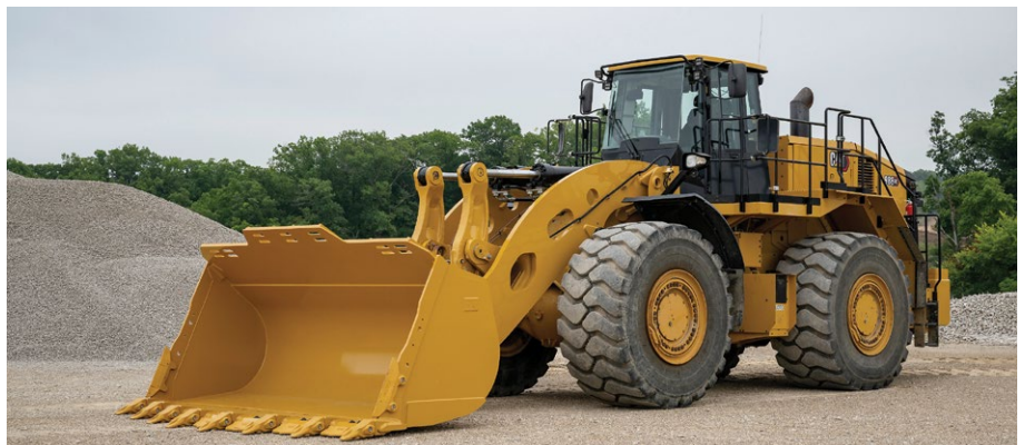
The new 988 GC is optimised as a 45-tonne (50-ton) truck match loader.
