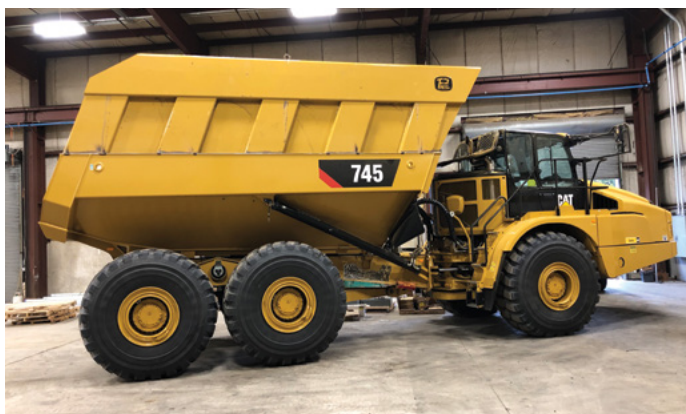
Sideboards are available in 2.54-centimetre increments from 15.24 centimetres to more than 101.6 centimetres, depending on the haul truck, the environment, and the material being hauled.
