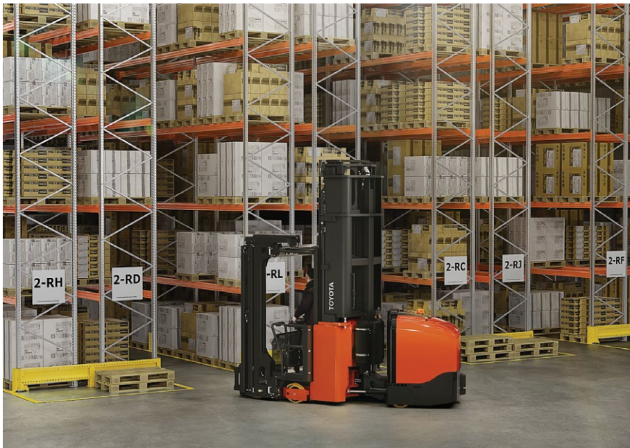
Lithium-ion batteries allow intermittent charging, reducing downtime and maximising equipment availability.
