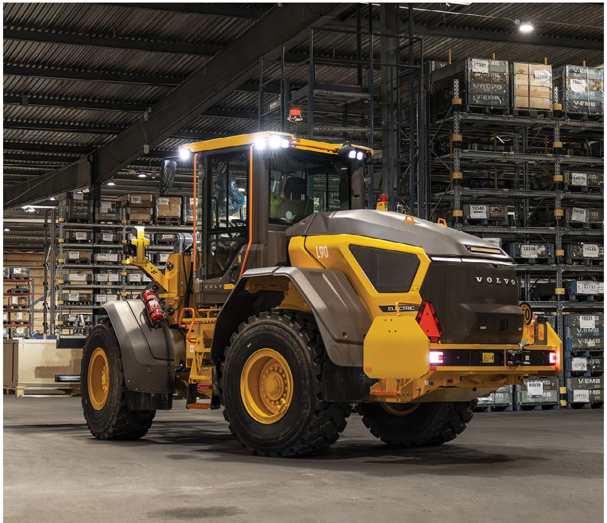
The first electric wheel loader in its class, the 15-ton L90 Electric is a multi-talented solution suitable for a wide range of jobs.
