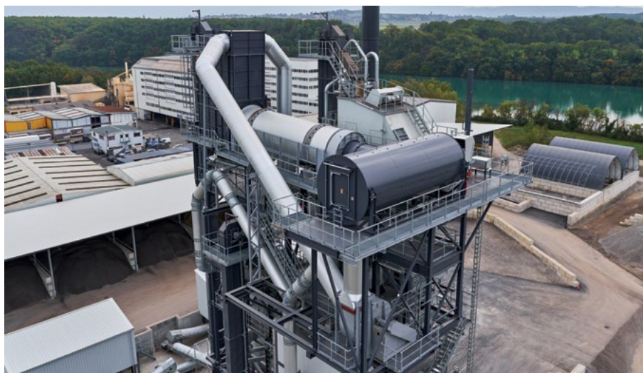
Benninghoven plant with a hot gas generator for asphalt production from up to 100% milled material.
