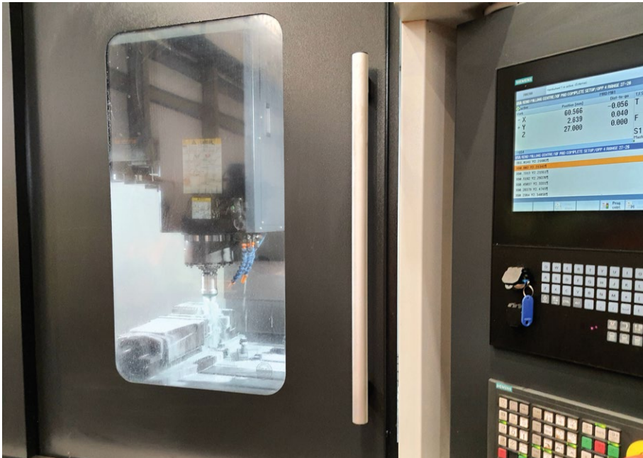
At the site, there's a CNC vertical machining centre, which allows the facility to produce its own aluminium mould inserts to produce polyurethane screen media.
