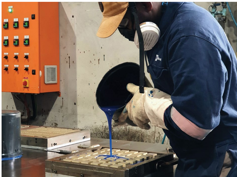
Open cast pouring is used at the FLSmidth Delmas manufacturing facility to manufacture panels.
