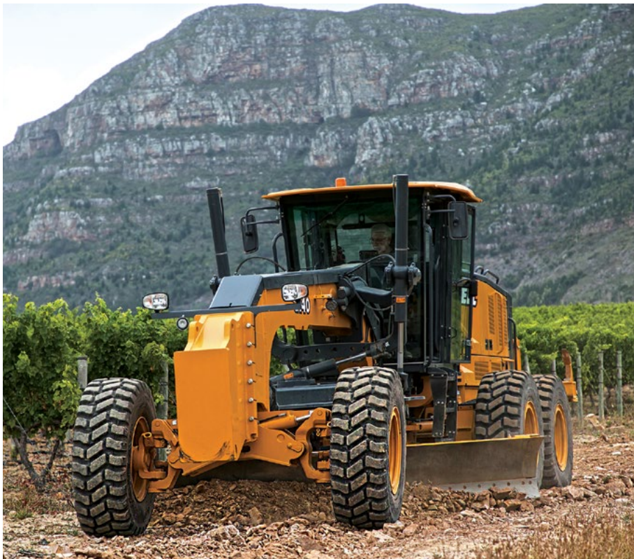
Automation has been one of the significant drivers in the motor grader design process to allow the operator to be more focused on the job at hand and the final product of his grade while still improving fuel efficiency and component life expectancy.
