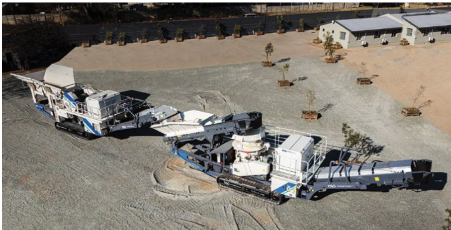
The electric Powertrack range, manufactured by SRHeavy (SRH) - a Metso-owned company, comprises mobile jaw crushers, cone crushers, and screens powered entirely by an external power supply.
