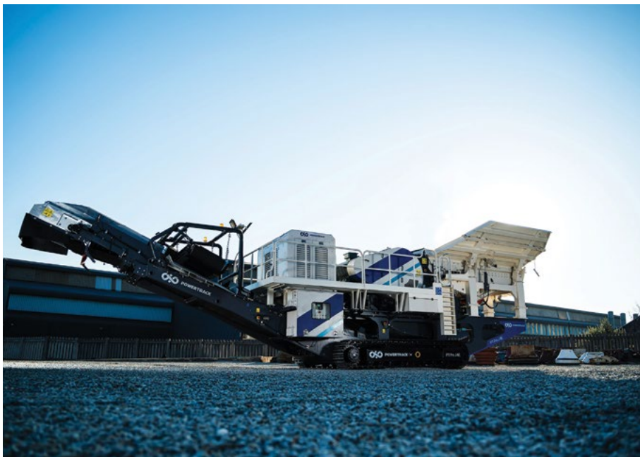
The Powertrack PT PRO J-11E mobile jaw crusher is equipped with a 1060 mm x 700 mm jaw crusher, vibrating feeder, overband magnet, dust covers and a discharge hood.
