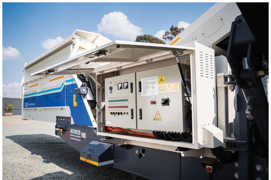
High-capacity material separation is achieved with the Powertrack PT Pro ST-08E triple-deck screen, powered by a fully electric drive.
