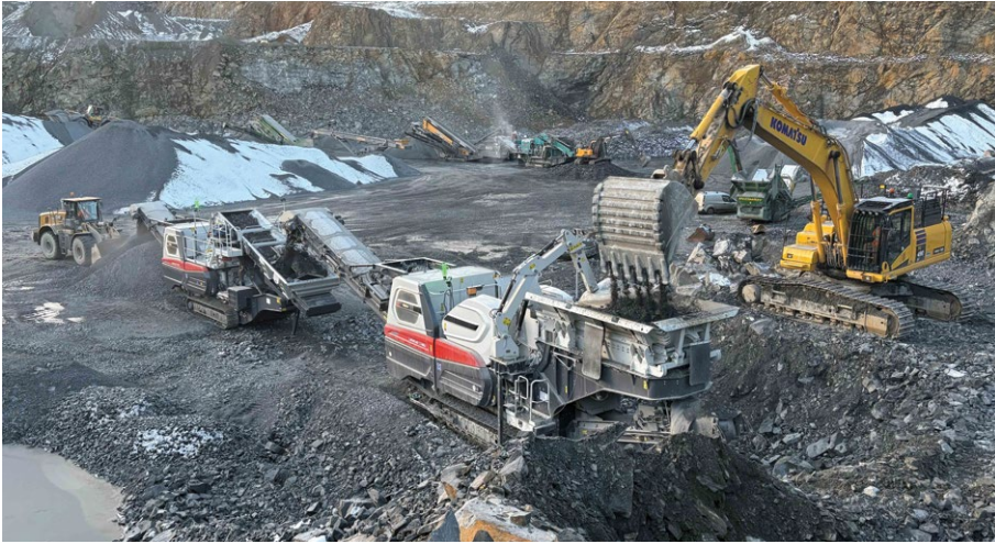
The Metso Lokotrack LT400J introduces a new generation of high-capacity, diesel-electric primary crushing technology to Africa.
