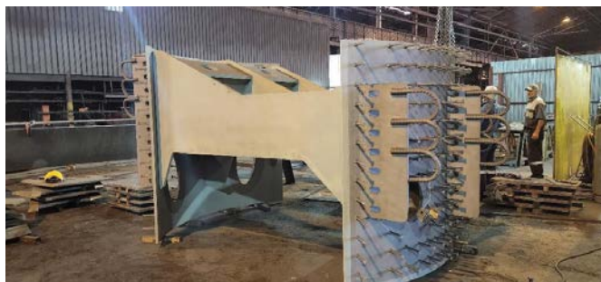
Left: Msikaba Bridge construction (October 2023). Right: Typical pylon liner under fabrication (June 2023).
