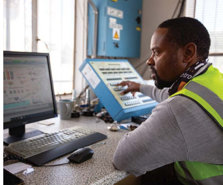
Left: AfriSam also prioritises the use of recycled water in its readymix plants. Right: AfriSam's batching plants use computerised batching systems to ensure compliance with mix designs.
