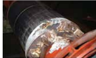
Image 6: Aluminium rotor stalled overheating.
