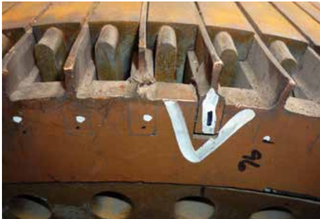
Image 16: Poor Brazing and fractured bar.
