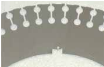
Image 4: Typical double cage rotor punching.
