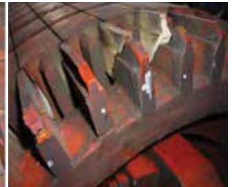
Image 11: Fractured rotor bars.
