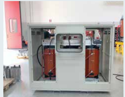
A specialised outdoor application transformer with special protection against water and solid objects.
