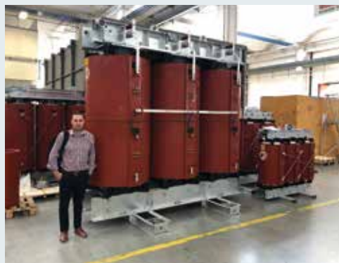
David Claassen, Managing Director of Trafo Power Solutions, in front of a 10 MVA cast resin transformer, ideal for high power demands.
