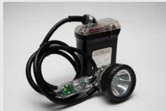
A RFID tag installed on pedestrians' cap lamps alerts them when they enter a danger zone.
