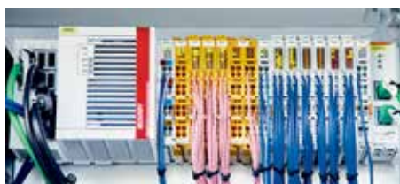
The CX5130 Embedded PC and the I/O level with EtherCAT and TwinSAFE terminals are very compact.
