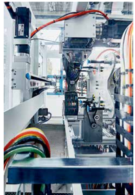
Two of the machine's four AM8000 servomotors move the main arm (motor on the right) and the shuttle (motor on the left).
