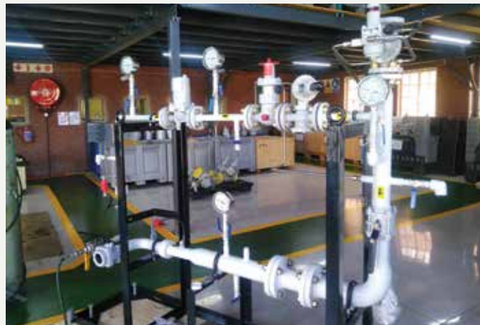
The skid-mounted high-pressure gas metering station was shop fabricated and assembled, fully tested and packaged before being transported to site.
