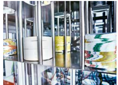
In each processing step, the IML system takes six labels at a time from a magazine and places them into the open mould of the injection moulding machine.
