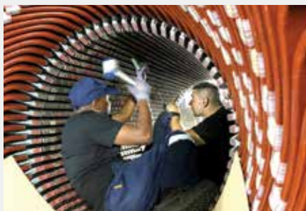
M&C undertook the repairs to a large 36MW compressor motor stator at Sasol's Secunda plant.
