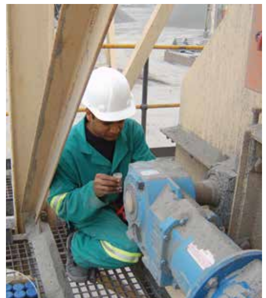
Taking an oil sample for testing; oil analysis is a critical element of WearCheck's transformer condition monitoring programme.
