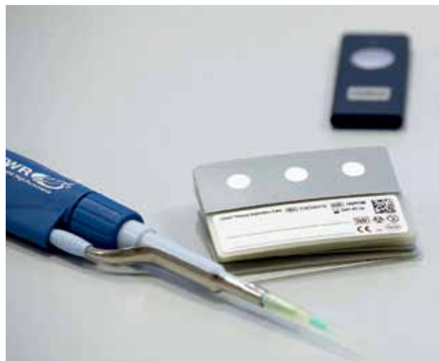
The Cobas PSC consists of a carrier layer with the bonded nonwoven fabric and an upper layer for protection and labelling.
