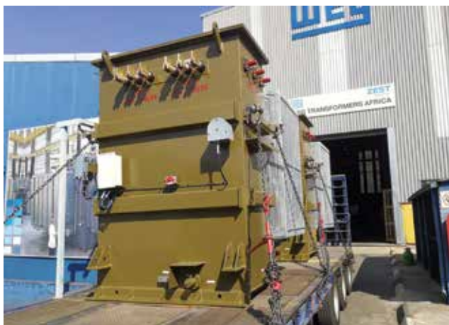
Two WEG PV transformers leaving the manufacturing facility to be delivered to site.
