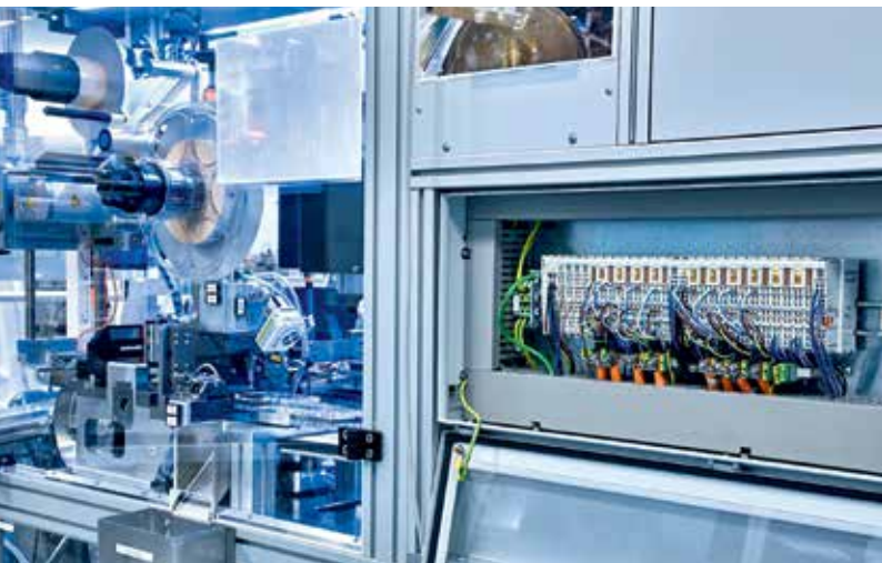
The EL7211 servomotor terminals (right) ensure precise motion sequences involving multiple axes in a particularly compact way.
