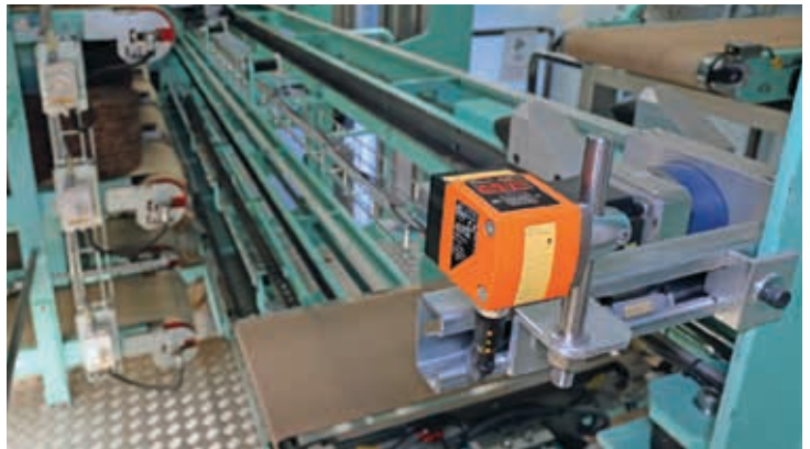
Above: The O1D sensor with time of flight technology enables position detection across longer distances.
