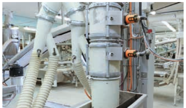
Capacitive sensors detect the flour through the walls of the pipes.
