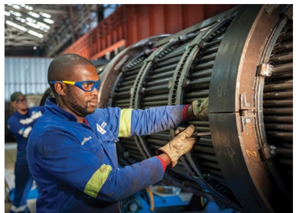
Final fitments on a high-pressure heater tube bundle before the shell is placed over it.
