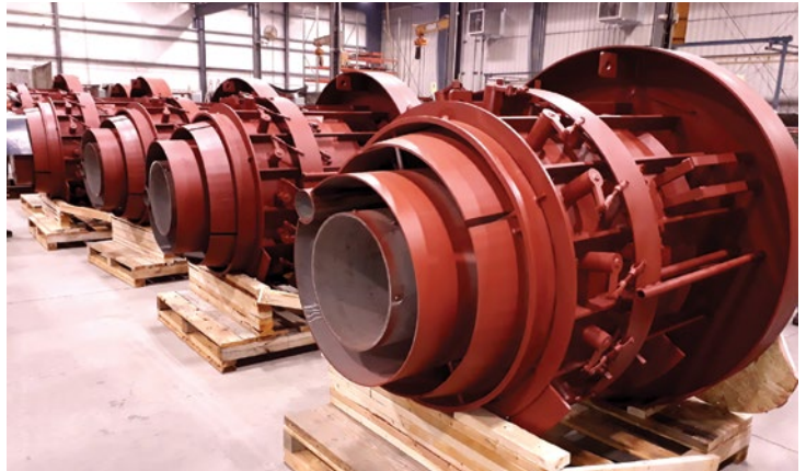
The low NOx burners fitted to pulverised coal-fired boilers have reduced NOx emissions significantly.
