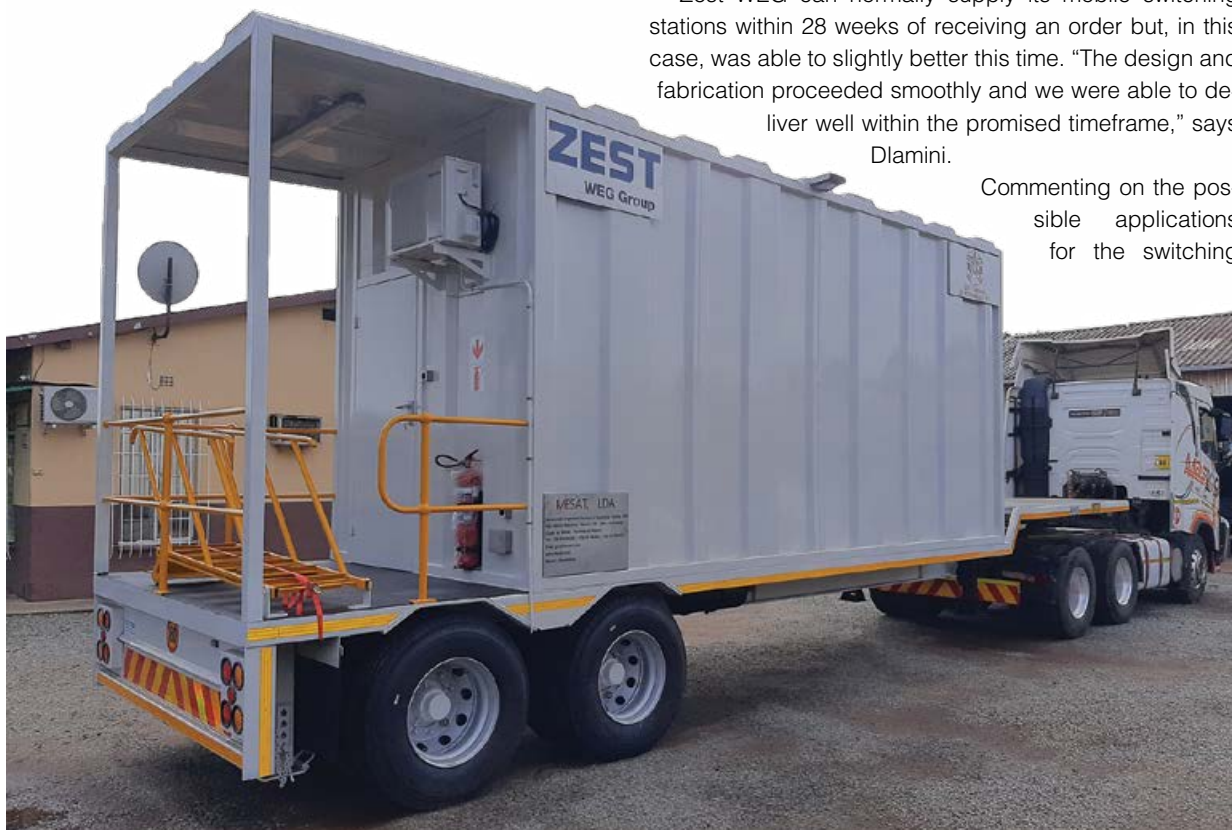
The 33 kV mobile switching station is ideal for routine maintenance or as a temporary stand-in when an existing station has failed.
