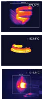
The Optris PI 1M IR camera provides for fast temperature measurement.
