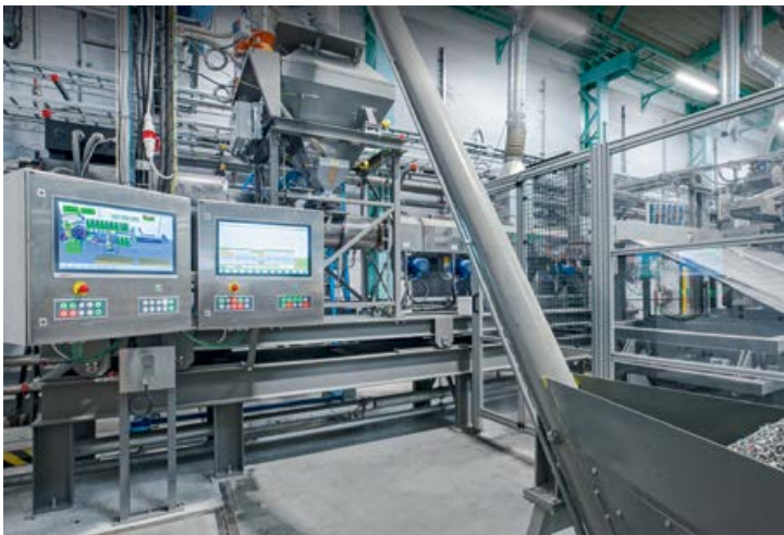
Govaerts integrates the messages from the EL9227 electronic overcurrent protection terminals into the HMI on its recycling machines.
