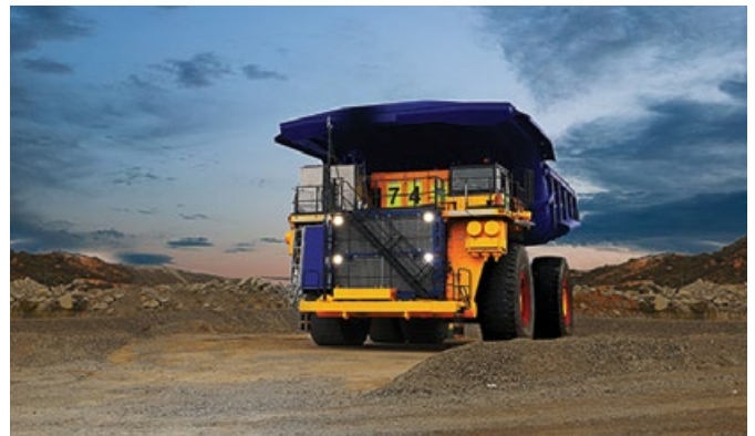
The 2 MW hydrogen-battery hybrid haul truck has a 290-tonne payload.
