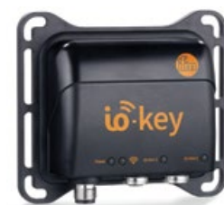
The io-key transmits the measured values of connected sensors with IO-Link interface directly to the cloud via the mobile network.
