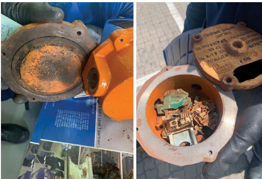
The photographs show the environmental effects on a flameproof junction box.
