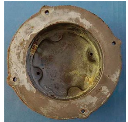
Left: Corrosion of a flame path on a cast iron junction box after testing to ASTM B117-03 and ISO 6988 standards. Right: A good quality flameproof junction box which has been specially treated with a corrosion-resistant metallurgical process after testing to ASTM B117-03 and ISO 6988 standards.
