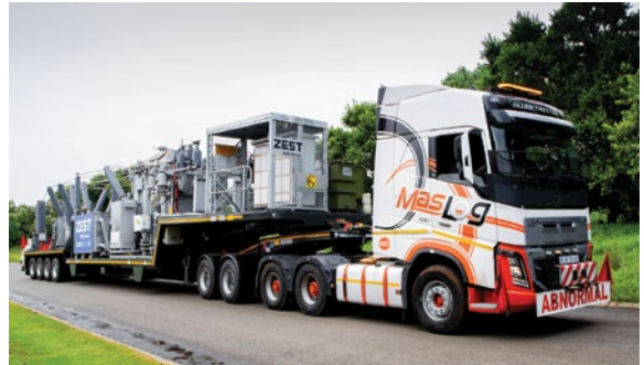
The 50 MVA mobile substation, which includes a dual voltage rated transformer, will be commissioned on-site early in 2022.
