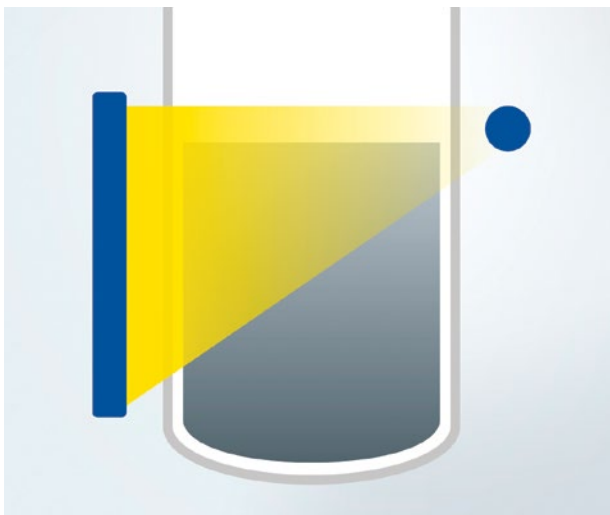
Rod source with point detector arrangement.
