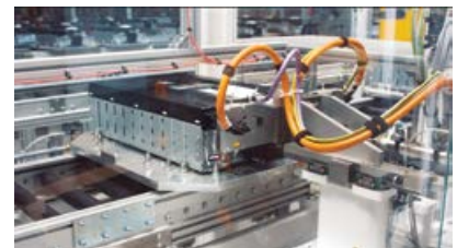
End-of-line testing of a battery module at Tesvolt's Gigafactory.
