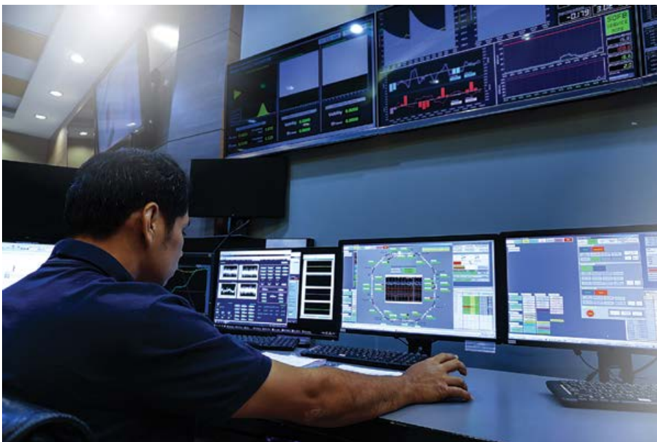
The Valmet D3 interface displays real-time process information in a customer-oriented graphical HMI.
