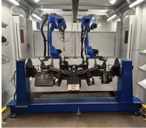
In each welding cell, two GP25 robots run in synchronised motion with a set of positioners, all housed in a protective enclosure.
